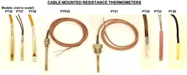
PT30 - Ø6mm, cable lead PT37 - Ø4 or 3mm, wire leads PT38 - with the hole for a bolt insulating jacket PT35 - adjustable collet nut PT31 - firmly welded nut Ø4.2 PT34 - in teflon sleeve (low price) PT33 - flat design (to be mounted in a motor groove) PT36 - embedded,
