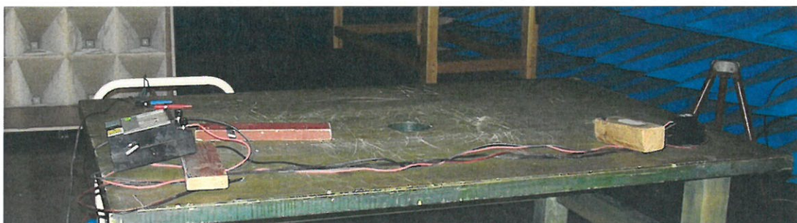
Fig.3 Arrangement of the EUT during the test according to EN 61000-4-3
