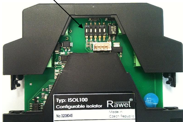
Setting DIP switch range selection.
