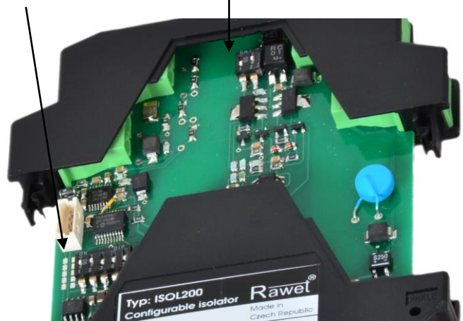
Setting DIP switches range selection.
